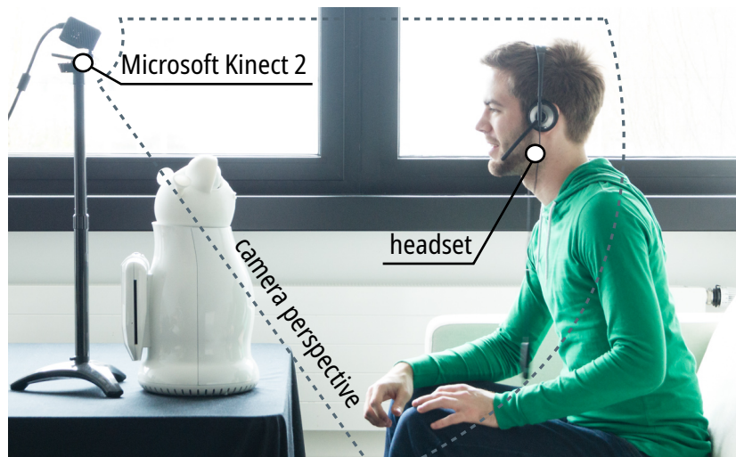
Figure 14.3.: Social signal processing is based on a Microsoft Kinect 2 sensor for posture estimation and a headset for speech recognition.
