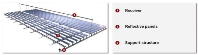
Figure 2-6: The LFR main components [49].
