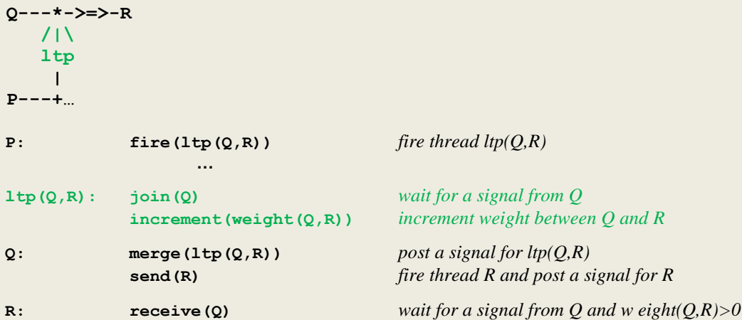
Figure 4. Micro-circuit and virtual machine instructions for ltp .
