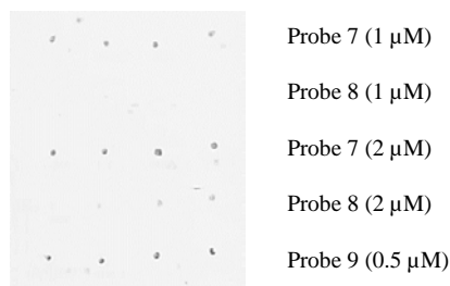
Figure 7. The absorbance signal obtained for the selective recognition of the PCR-amplified DNA samples of Salmonella using specific capture Probe 7 (1 and 2 \mu\text{M} ), Probe 8 (1 and 2 \mu\text{M} ) as the
