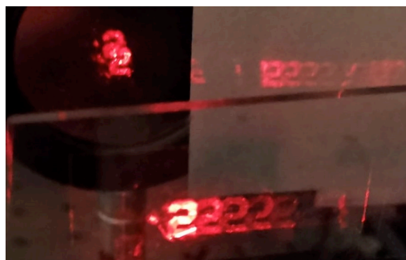
Figure 2. See-through system based on photopolymers working with red light
