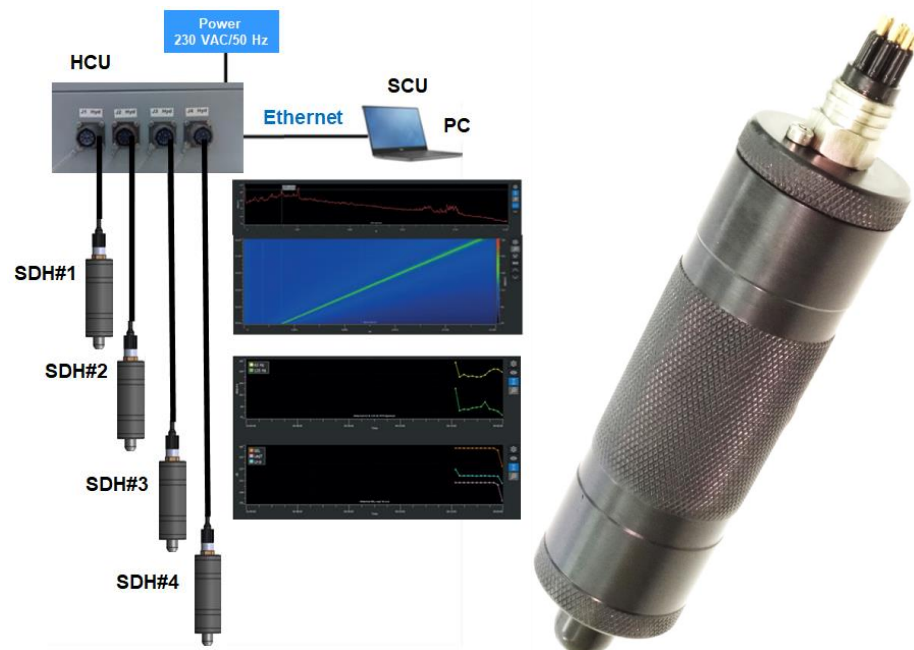
Figure 3. General architecture of the SDH system (left) and smart digital hydrophone (right). Image property of Sociedad Anónima de Electronica Submarina S.M.E. (SAES).
