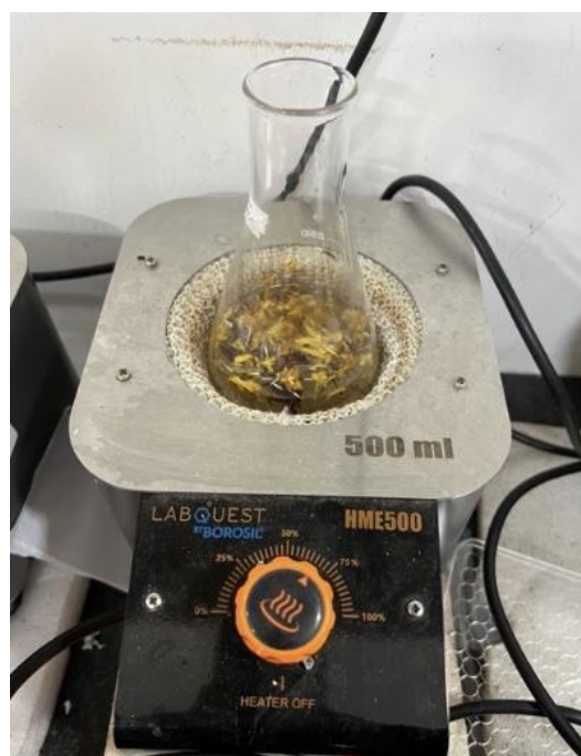
Fig 1: This figure shows Dry marigold and Dry hibiscus is heated under conventional heating at 80°C in an aqueous solution.
