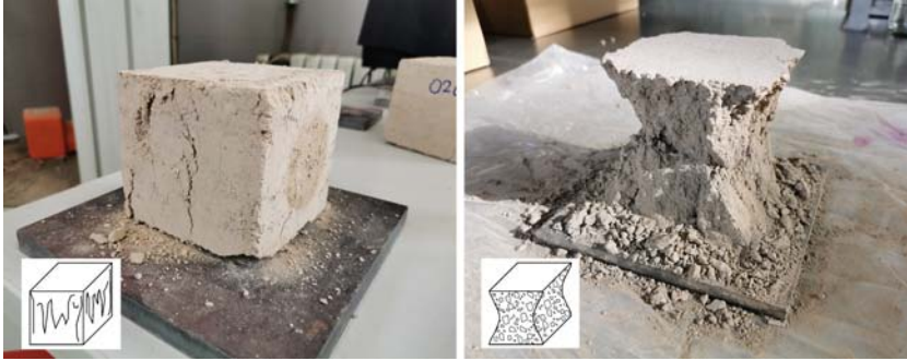
Figure 5.4: Satisfactory failures of cubic specimens, according to EN 12390-3 [209].
