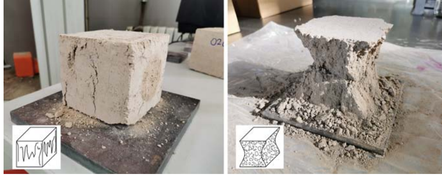
Figure 4: Satisfactory failures of cubic specimens, according to EN 12390-3 [52].
