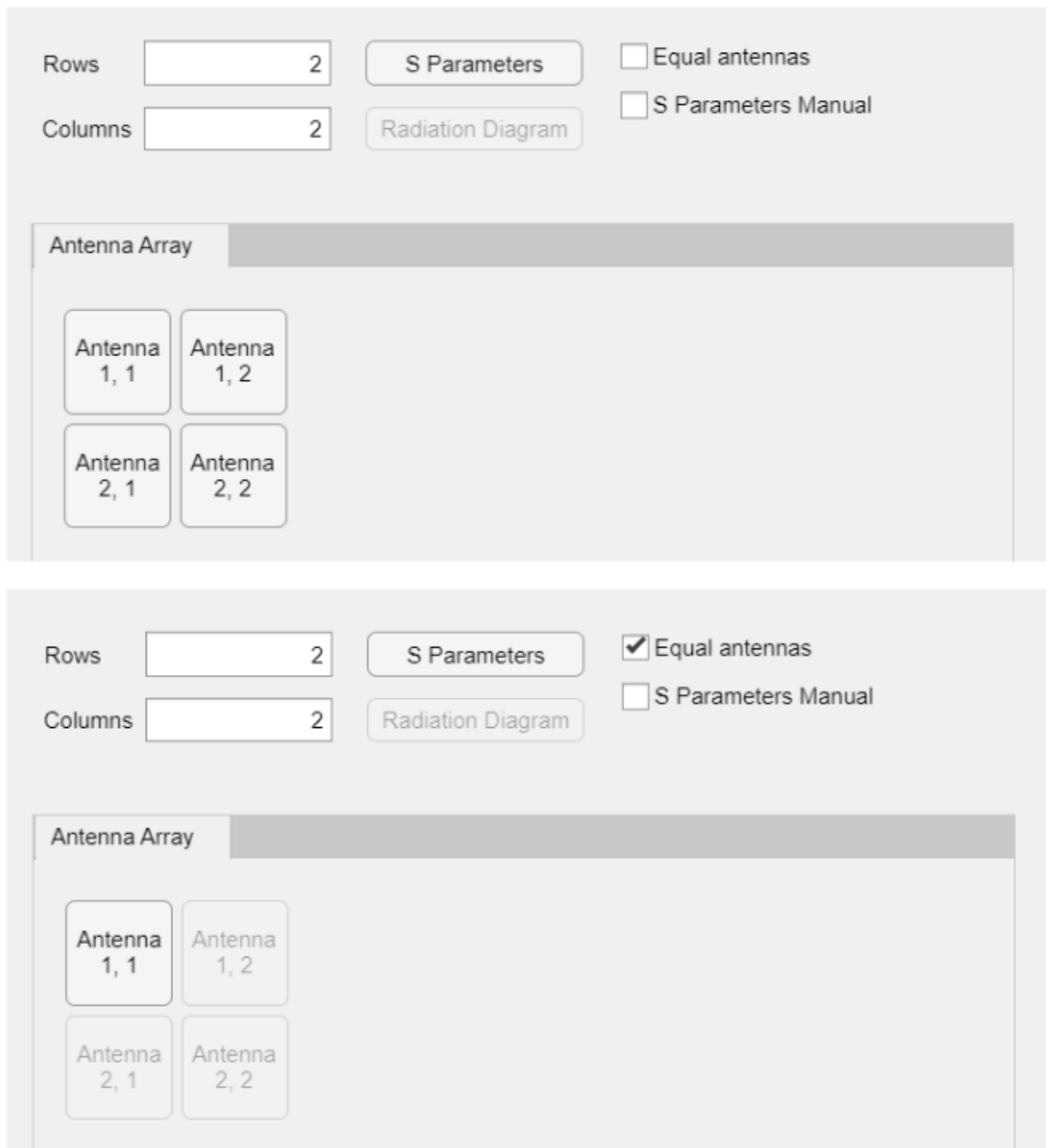
Figure 4.2: In the top image, the Equal antennas checkbox has not been selected, so all buttons are enabled. When it is selected, as it is possible to see in the bottom image, only the first button is enabled.
