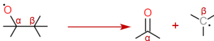
Figure 2.5: The mechanism of alkoxy bond scission. As shown in the figure, the carbon atom bonded to the alkoxy radical is referred to as the \alpha -carbon, whereas the carbon atom receiving the radical after the scission is referred to as the \beta -carbon.
