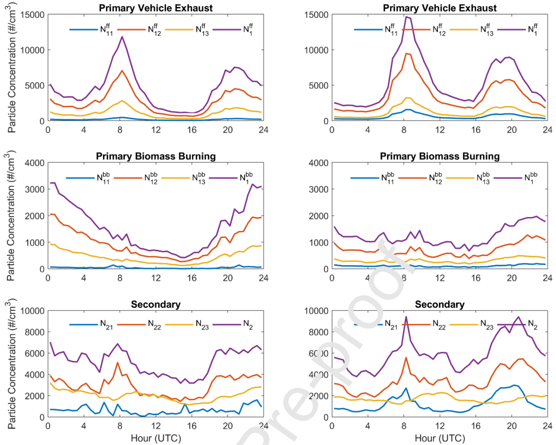
Figure 6. Diurnal evolution of mode segregated and total particle number concentrations from primary vehicle exhaust, primary biomass burning and secondary origin at suburban (left column) and urban sites (right column). N_{11} , N_{11}^{ff} , N_{11}^{bb} and N_{21} are the concentrations of total primary, primary vehicle exhaust, primary biomass burning and secondary particles in the 12-25 nm size range, respectively. N_{12} , N_{12}^{ff} , N_{12}^{bb} and N_{22} and N_{13} , N_{13}^{ff} , N_{13}^{bb} and N_{23} are the corresponding concentrations in 25-100 nm and 100-600 nm size ranges, respectively.
