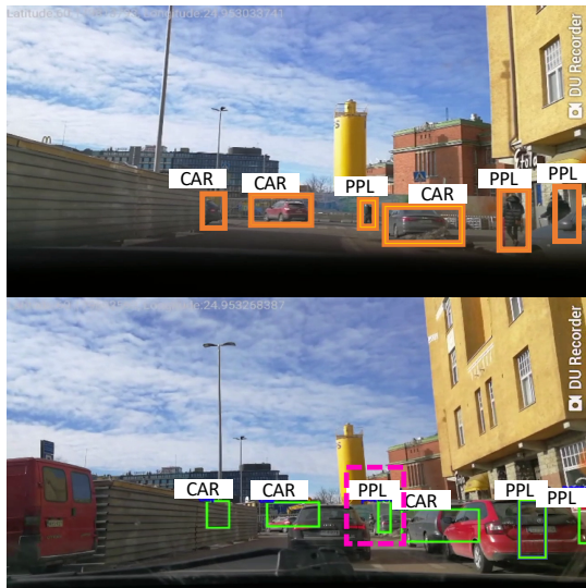
Fig. 1: Illustration of a naïve cooperative perception system. A leading vehicle detects objects shown in orange bounding boxes (top figure). These objects are displayed to the driver of the following vehicle in green bounding boxes (bottom figure). AICP filters such objects to only show critical ones (e.g., the pedestrians in the pink bounding box) to reduce on-screen object overload.
