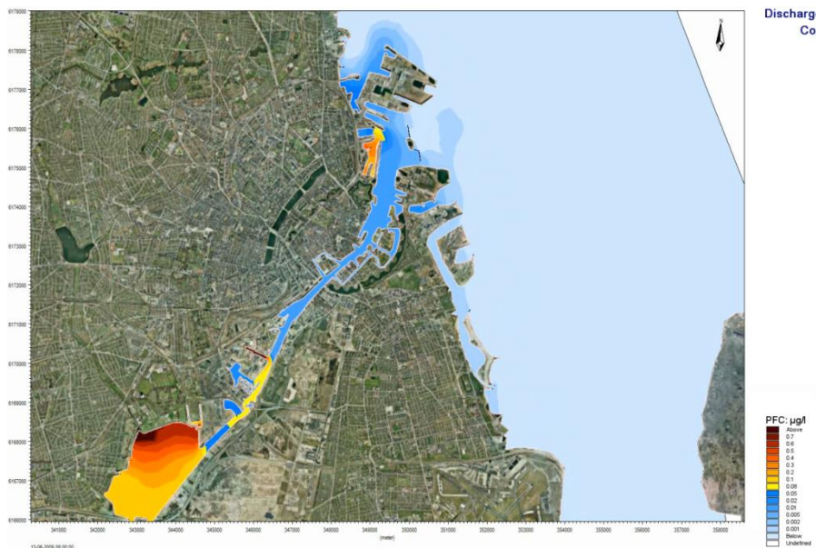
Figure 33: Hydrodynamic fate modelling of PFC in Copenhagen Harbour. The map illustrates the predicted situation after heavy rain in June 2009. This is a picture from the video animation, which can be viewed at www.cohiba-project.net .
