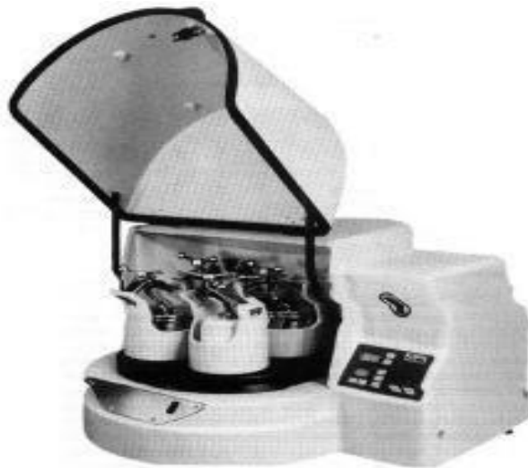
Figure 2. 10 Fritsch Pulverisette P-5 four station planetary ball mill (Neikov, 2019)
