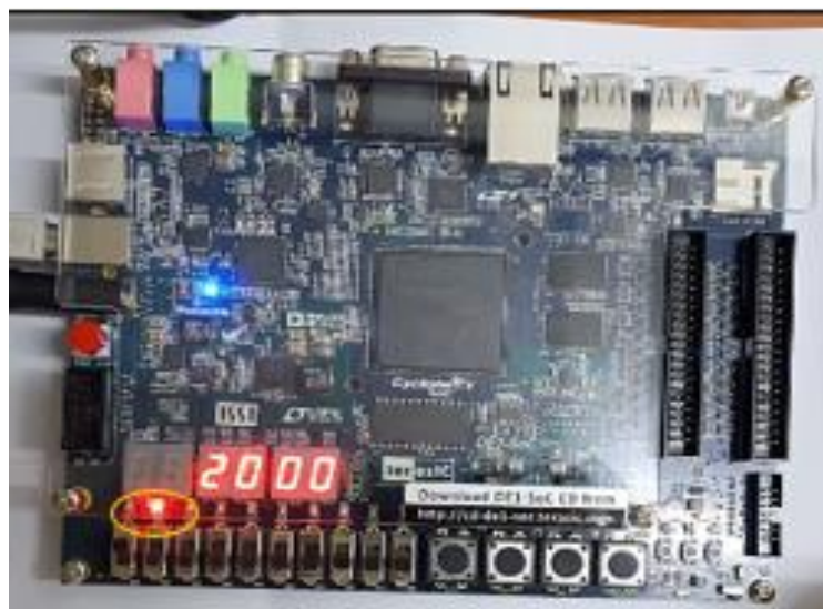
Figure 8. CUT-3 is tested with BIST scheme on FPGA
