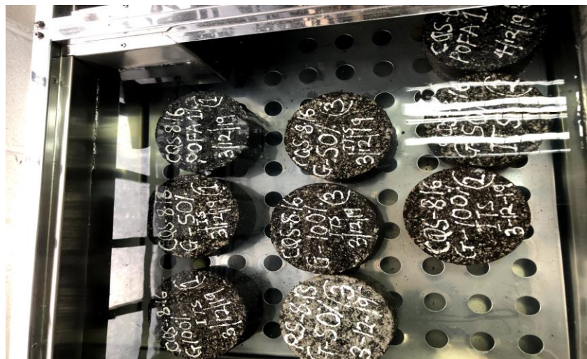
Figure 2. Moisture-conditioned samples in water bath at 60 °C.
