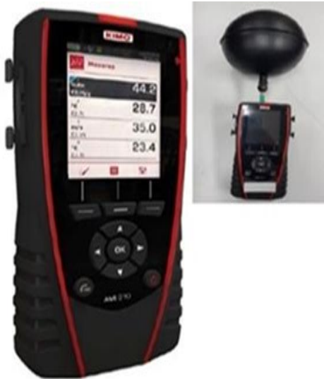
Fig. 10. KIMO instruments model AMI 310 with black globe
