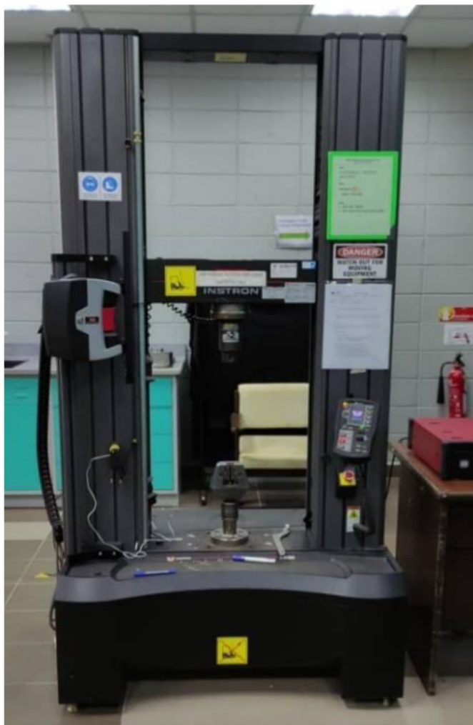
Fig. 6. Universal testing machine used to carry out quasi-static indentation test.
