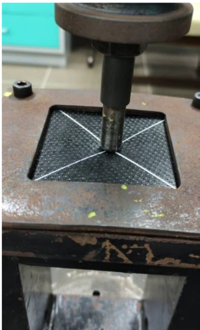
Fig. 9. Hemispherical indenter aligned with center of carbon/ramie fiber reinforced epoxy hybrid composite loaded to fixture.
