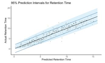
**Figure 2.** 95% prediction intervals (blue area) for the univariate MARS analysis on the square root of RT. Blue lines are placed at the predicted values  $\pm 2$  min. Approximately, only 8% of observed retention times were more than 2 min away from their predicted value.
