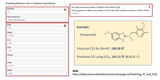
**Figure 4.** Online platform for the prediction of RT and CCS data using univariate models. (A) Selection of response to predict, that is, RT, CCS for (de)protonated molecules or CCS for sodium adducts; (B) introduction of molecular descriptors for the molecule of interest; (C) output of the predictor model together with the prediction intervals. Example illustrated by omeprazole.
