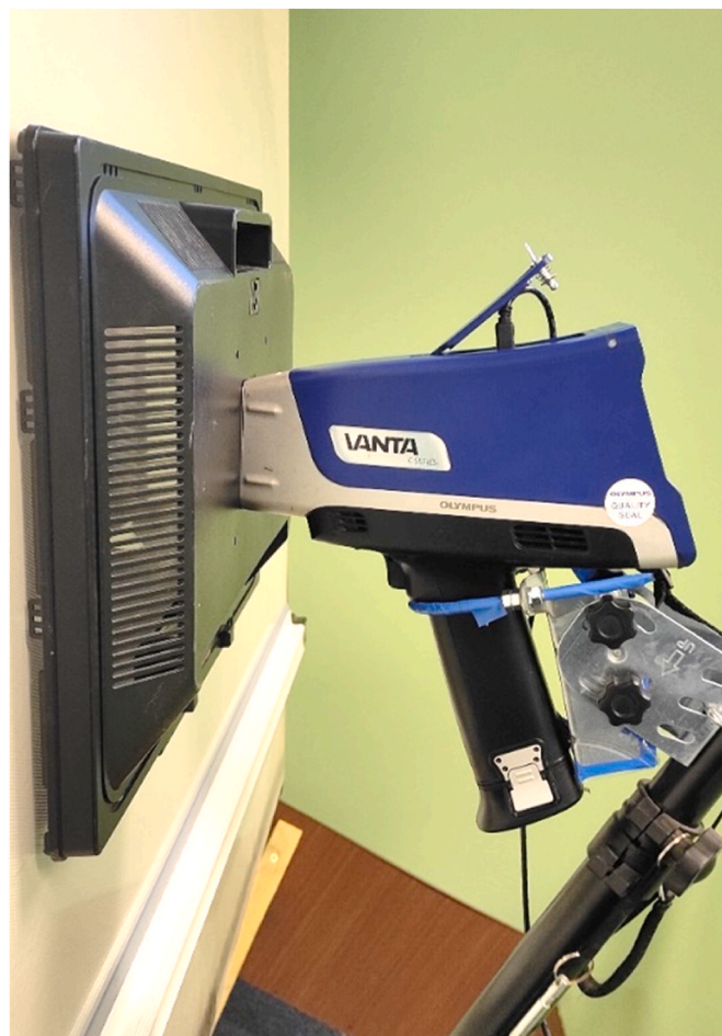
Fig. 1. 23" FPD plastic casing being analysed by the remotely operated VANTA™ handheld XRF Analyser (W: 8.3cm, L: 23.3cm, H:28.9 cm).
