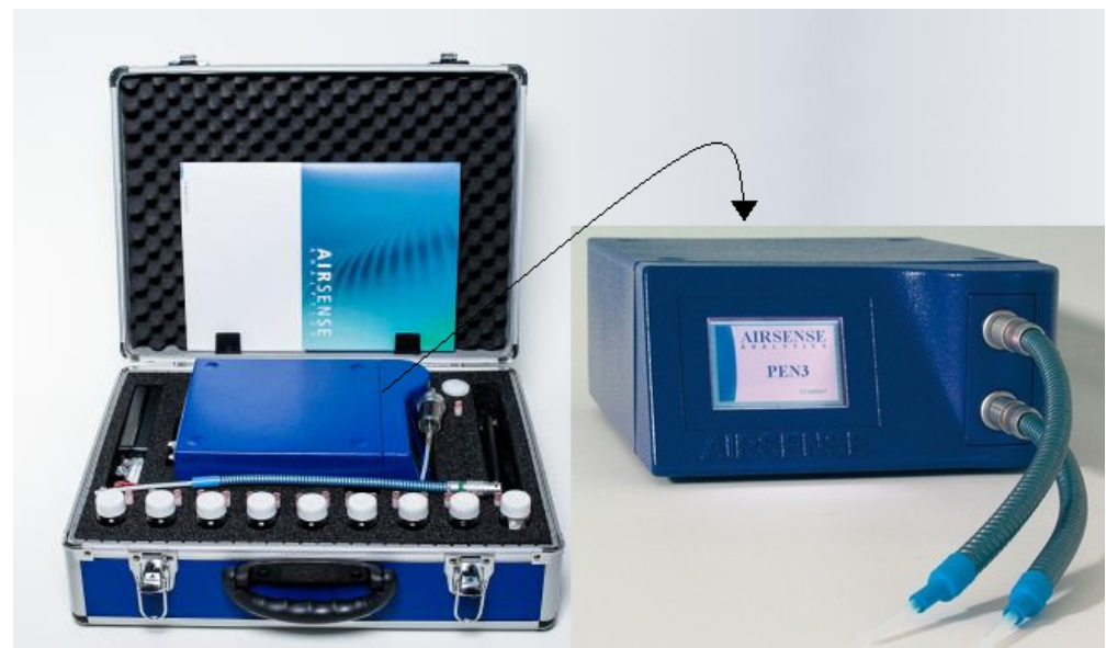
Figure 2. Portable electric nose version 3.5 (PEN 3.5).
