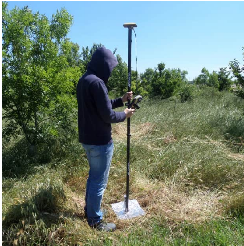
Figure 4. GNSS survey for a 0.3 \times 0.3 m GCP, in an area beside the cultivated fields.
