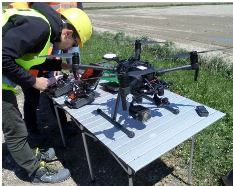
Figure 1. The UAV and payload selected for the AWL project is shown: DJI Matrice 210 with thermal and optical sensor.
