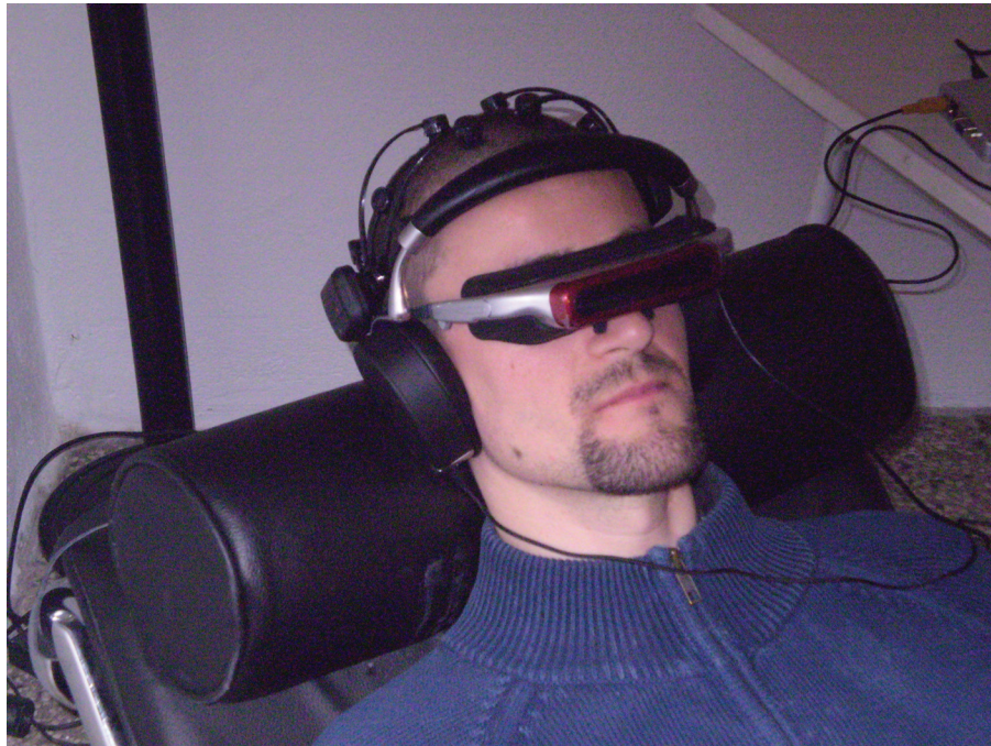
Figure S1. A participant wearing the complete apparatus used during the experiment: Emotiv™ EEG, digital glasses and headphones.
