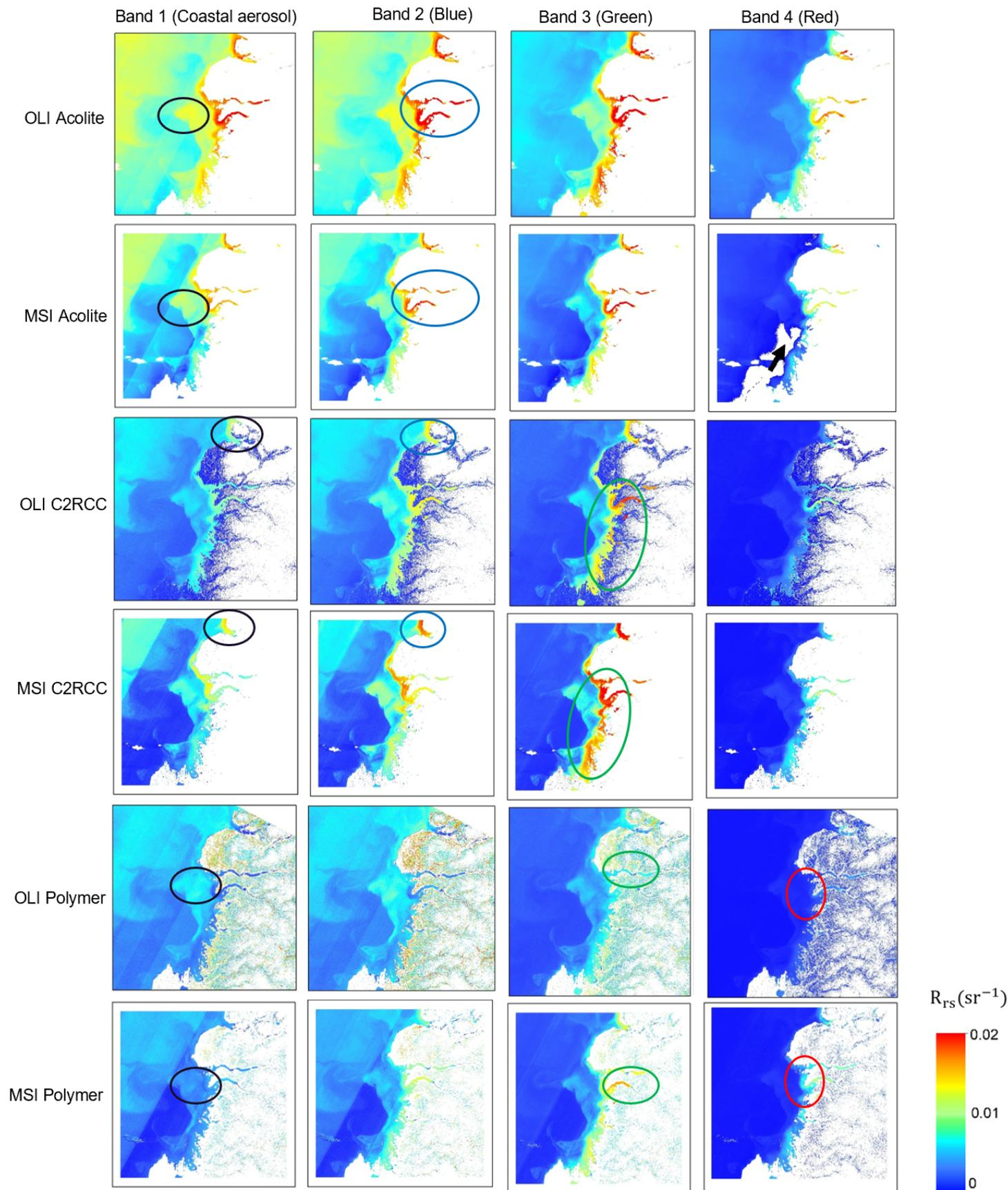
Fig. 9: Comparison between near-simultaneous OLI and MSI  $R_{rs}$  products derived via Acolite, C2RCC and Polymer, for the similar bands using the images shown in Fig. 8. The areas indicated by ellipses (colors matching the band number) highlight the similarities/differences in OLI-MSI  $R_{rs}$  products when processed via different AC schemes.
