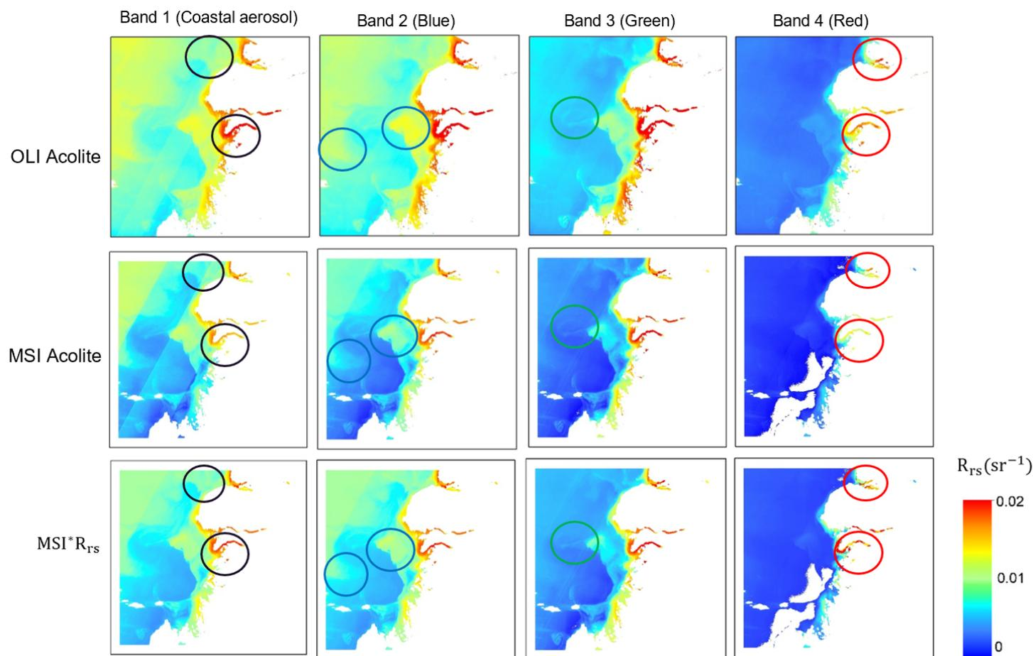
Fig. 10: Comparison between OLI, MSI, and  $MSI \cdot R_{rs}$  (after bandpass adjustment) products. The areas indicated by ellipses show that OLI produced higher/lower  $R_{rs}$  values compared to MSI. These differences in magnitude are minimized after applying the proposed BA model.
