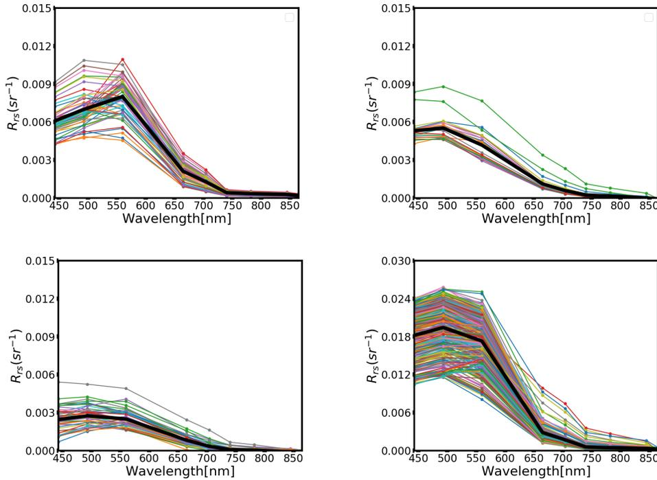
Fig. 4: In-situ  $R_{rs}$  spectra of the four match-ups with a time-difference of  $\pm 3$  hours with Sentinel-2 A/B overpasses, convoluted to the S2-MSI spectral bands using the Sentinel-2 A/B Spectral Response Functions S2-SRFs (version 3.0). The solid black lines refer to the mean  $R_{rs}$  spectra.
