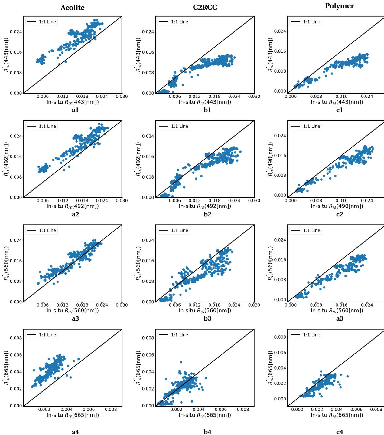
Fig. 6: Overall performance comparison of AC processors against the in-situ data in the four visible bands using data acquired from the S2 MSI. Detailed statistical metrics are available in Table. III. The solid black lines are the 1:1 match.
