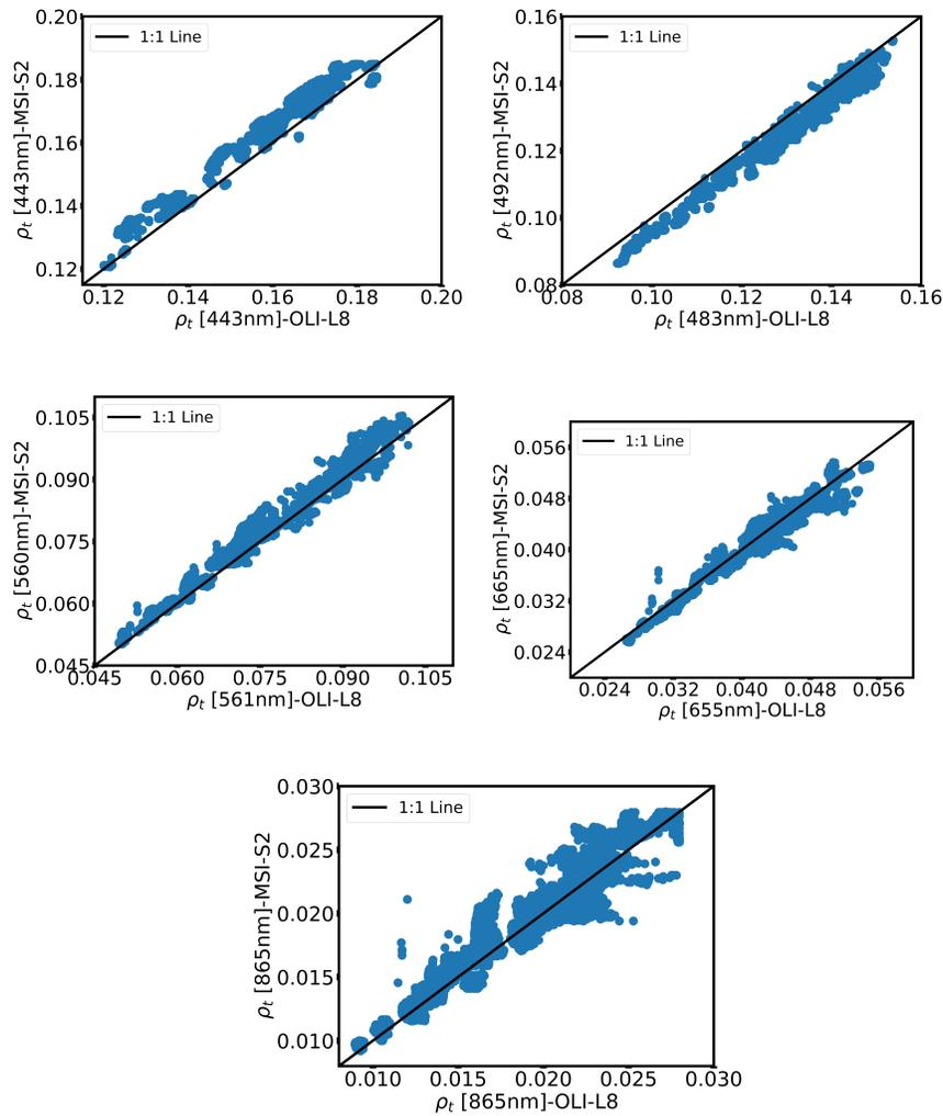
Fig. 11: Inter-comparison of TOA reflectance  $\rho_t$  products for L8-S2 pairs. Detailed statistical metrics are available in Table. V.
