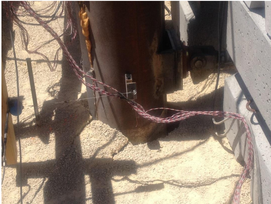
Figure 5.32: Cracking and heaving of soil in front of pile 3.1D.
