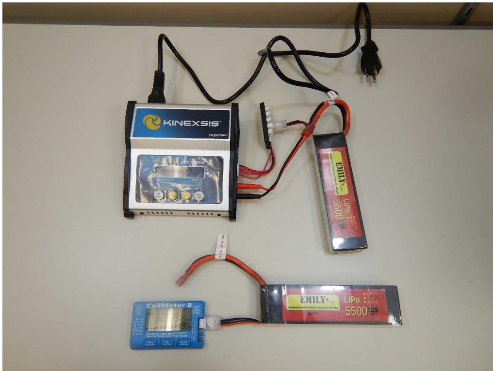
Figure 10: Battery Charging Set Up
