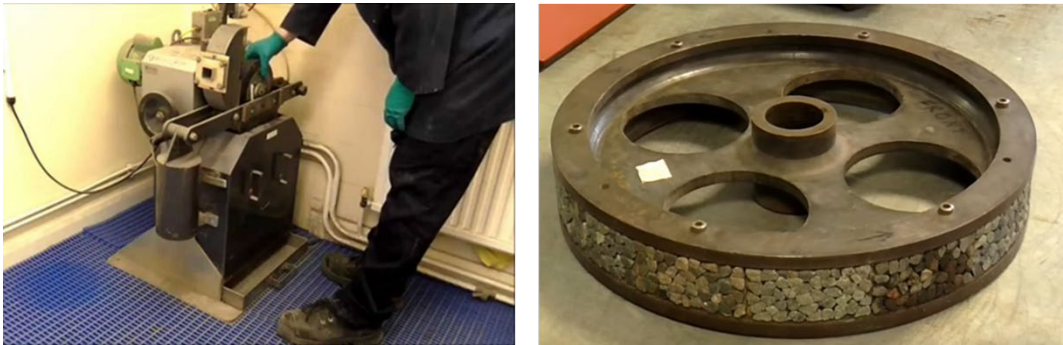
Figure 1.9 Accelerated polishing machine and aggregates (Roe and Hartshorne, 1998).
