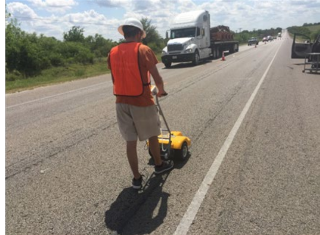
Figure 1.16 Micro-GripTester device (left) and field operation (right)
