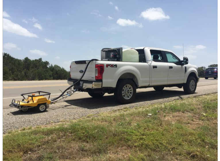
Figure 1.15 GripTester device (left) and field operation (right).
