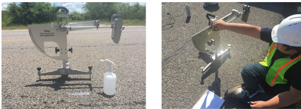
Figure 1.13 BPT (left) and field operation (right)
