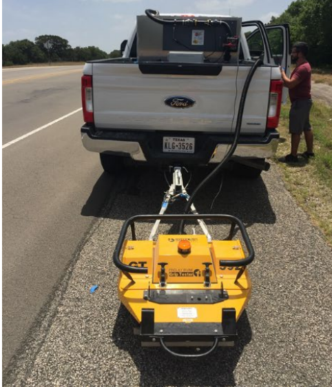
Figure 1.15 GripTester device (left) and field operation (right).
