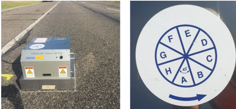
Figure 1.5 CTM (left), and CTM segments (right)
