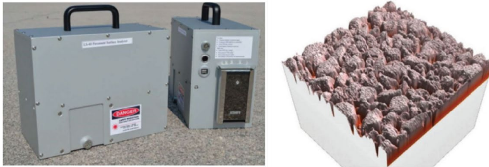
Figure 1.8 LS-40 Portable 3D Surface Analyzer (left), 3D surface scan (right) (Li et al., 2017)
