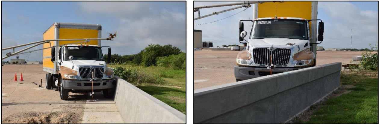
Figure 6.1. Barrier/Test Vehicle Geometrics for Test No. 469689-3-3.
