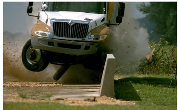
Figure C.1. Sequential Photographs for Test No. 469689-3-3 (Overhead and Frontal Views).
