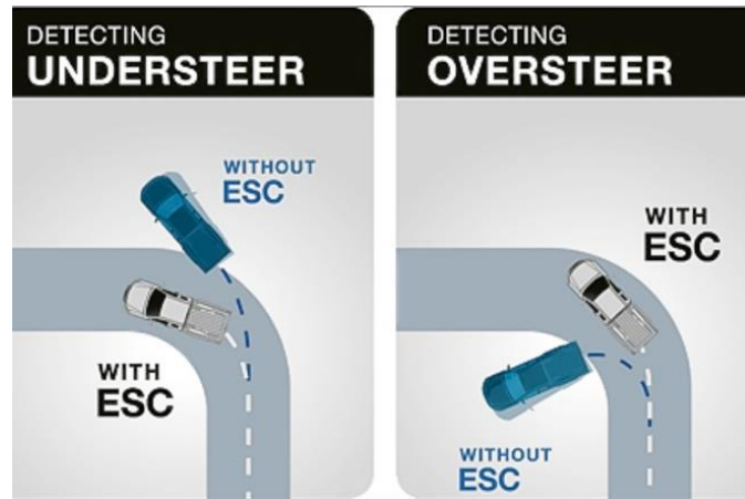
FIGURE 16 Electronic Stability Control (29)
