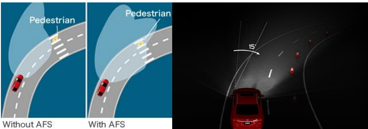
FIGURE 7 How Adaptive Front-Lighting System Works (16)
