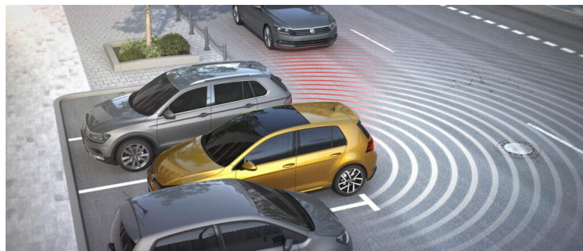
FIGURE 22 Rear Cross Traffic Alert (42)
