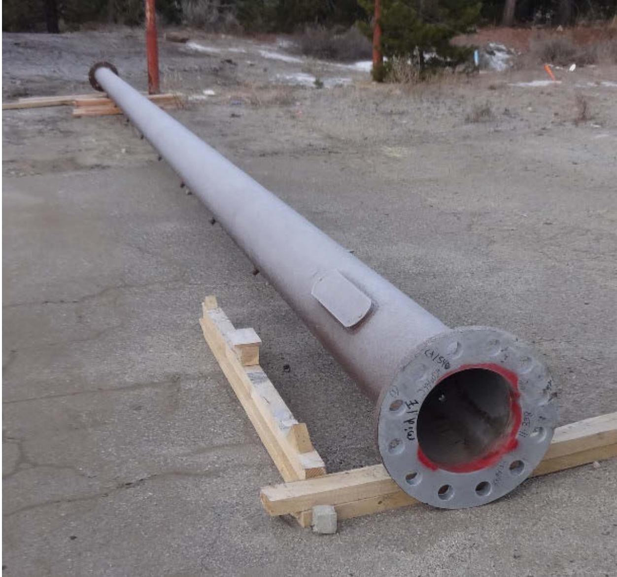
Figure 26. MG 2 Internal-Type Mounted Pole
