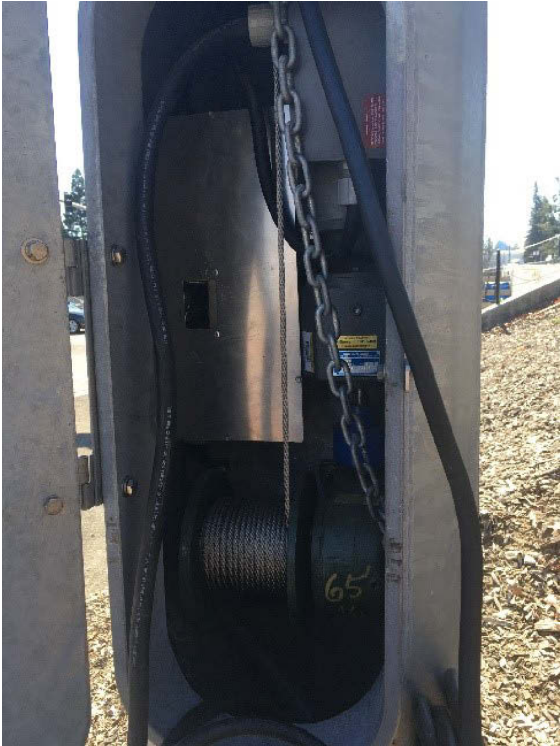
Figure 4. Stratus Internal Winch Tool with Integrated Electric Motor
