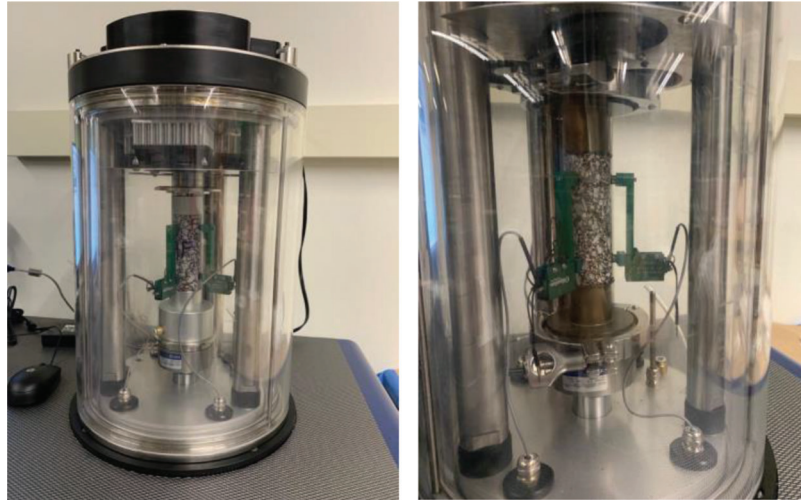
Figure 4.1 Dynamic modulus and cyclic fatigue test setups.
