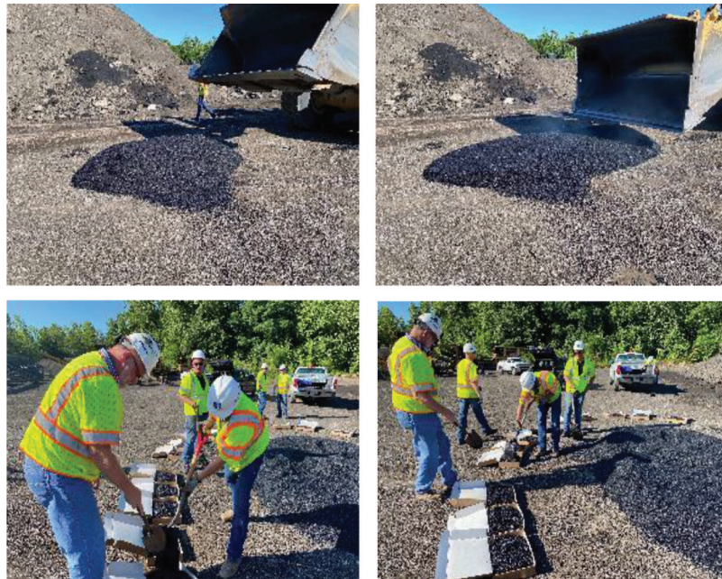
Figure 2.20 Process used to obtain plant-mix sample for the 9.5-mm surface mixture. Mixture was dumped from the silo into a truck, placed on the ground, flattened with a loader, and shoveled from random locations into boxes.
