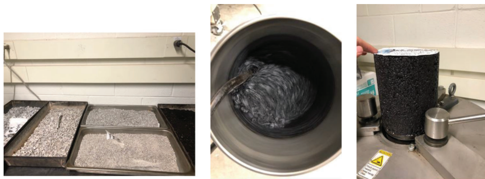
Figure 3.1 LMLC samples preparation: (a) aggregate pans, (b) mixer, and (c) SGC specimen.
