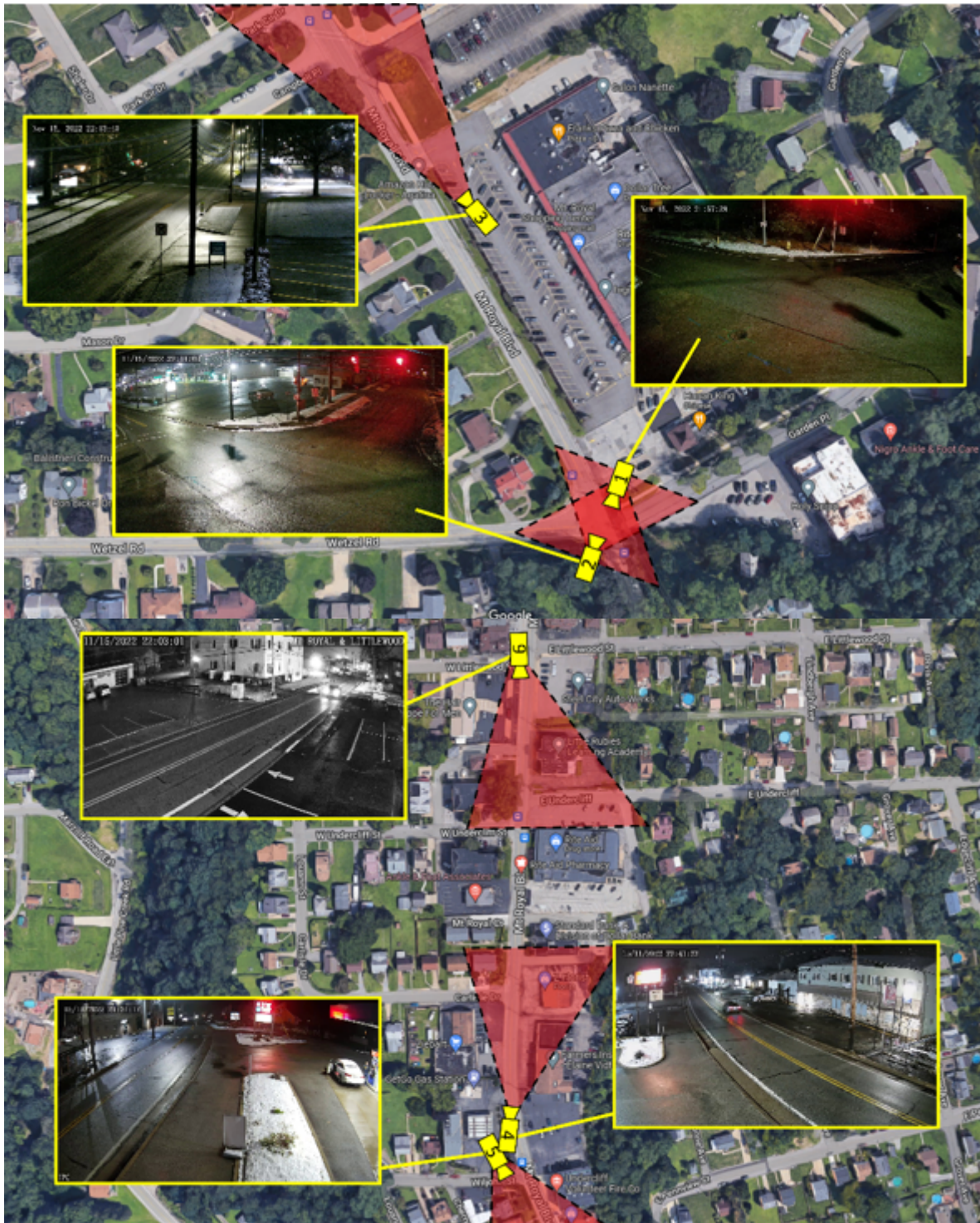
Figure 1: Location of 6 cameras that were installed along Mount Royal Boulevard. Each camera is illustrated with approximate viewing angle and field of view as shown in example image captures. Top: First 3 installed and Bottom: Last 3 installed cameras. (Source: CMU Robotics).
