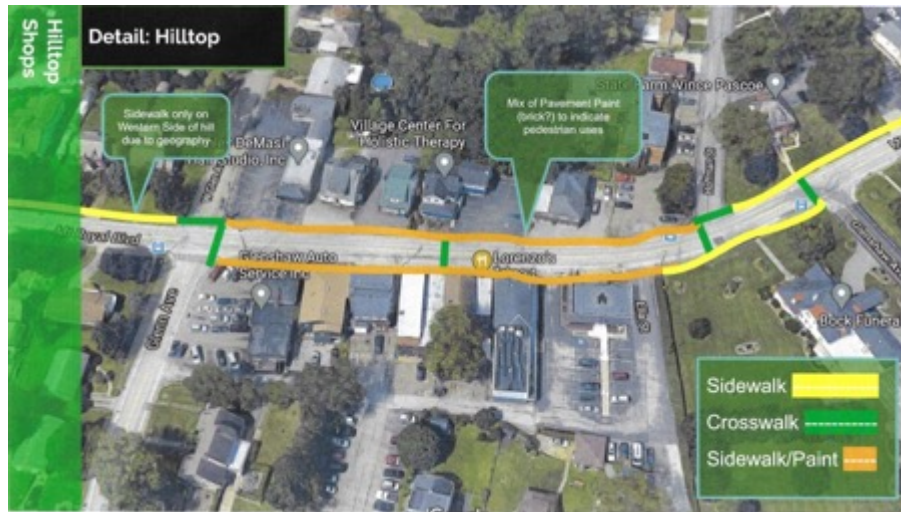
Hilltop Shops detail of a portion showing sidewalks identified by painted lines in curb cut locations in front of retail locations. (Source: Walk Bike Shaler).
