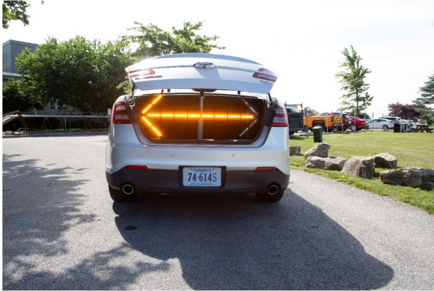
Figure 10. Lighting Display in the Trunk of the Following Vehicle
