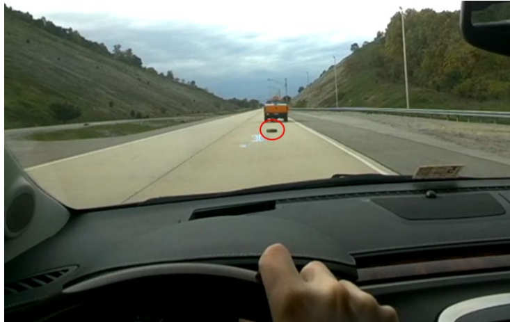
Figure 8. Participant Perspective of the Cardboard Box Dropped From the Lead Vehicle (Box Circled in Red)
