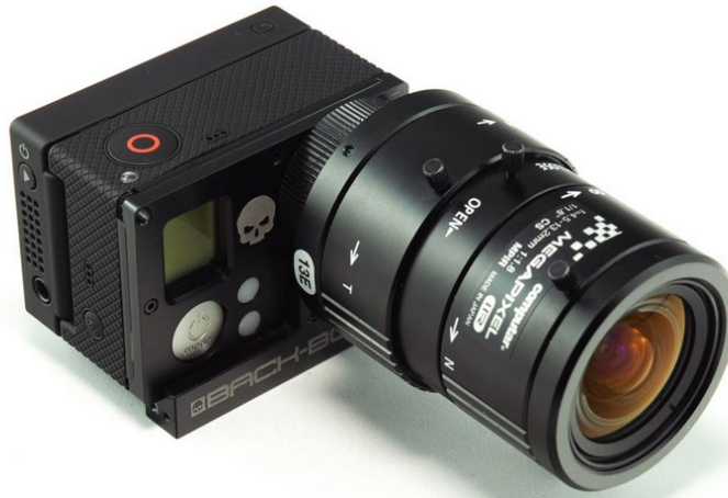
Figure 3. The Modified GoPro Camera With Attached Zoom Lens
