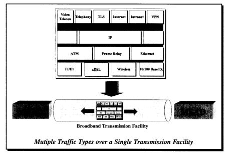
be an ATM or Frame Relay virtual circuit, an IP/Ethernet flow, etc., but it rides over a single transmission facility. This could be an existing T1 or DSL connection. Alternatively, it might be one of the newer broadband wireless technologies.
