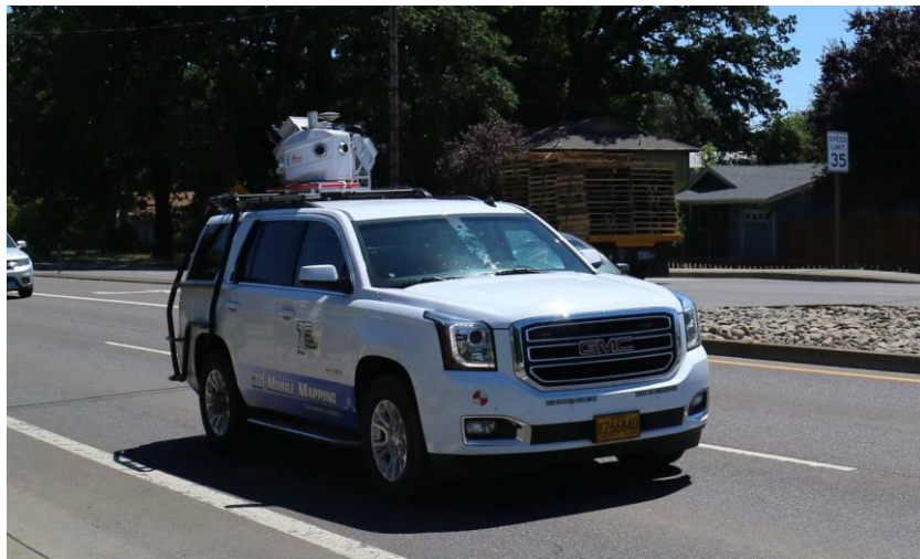
Figure 2.4 Mobile LiDAR System on a Moving Vehicle (Olsen et al., 2018)
