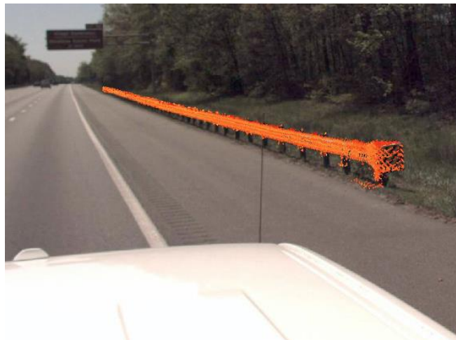
Figure 2.8 An Example of Guardrail Scan and Automatic Extraction by Pillar
