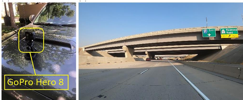
Figure 2.7 Mobile Photogrammetry Setup and the View (Farhadmanesh et al., 2021)
