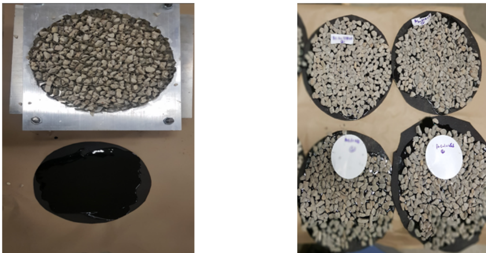
Figure 3.2. Specimen fabrication for the Sweep test (left: specimen before applying aggregates; right: after placing aggregates)
