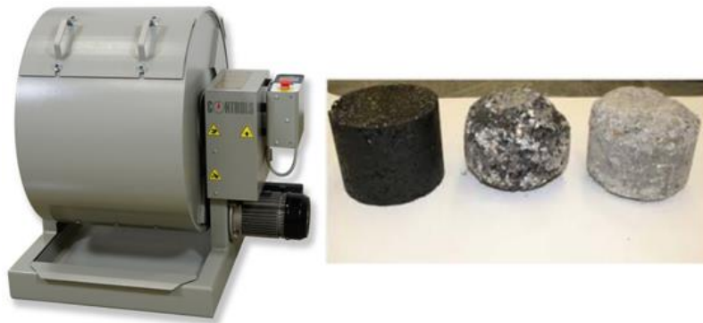
Figure 2.1. Cantabro Test Equipment (TEX-245-F, 2019)
