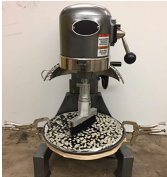
Figure 2.2. A photograph of the Sweep test shown with the brush attachment (ASTM International)
