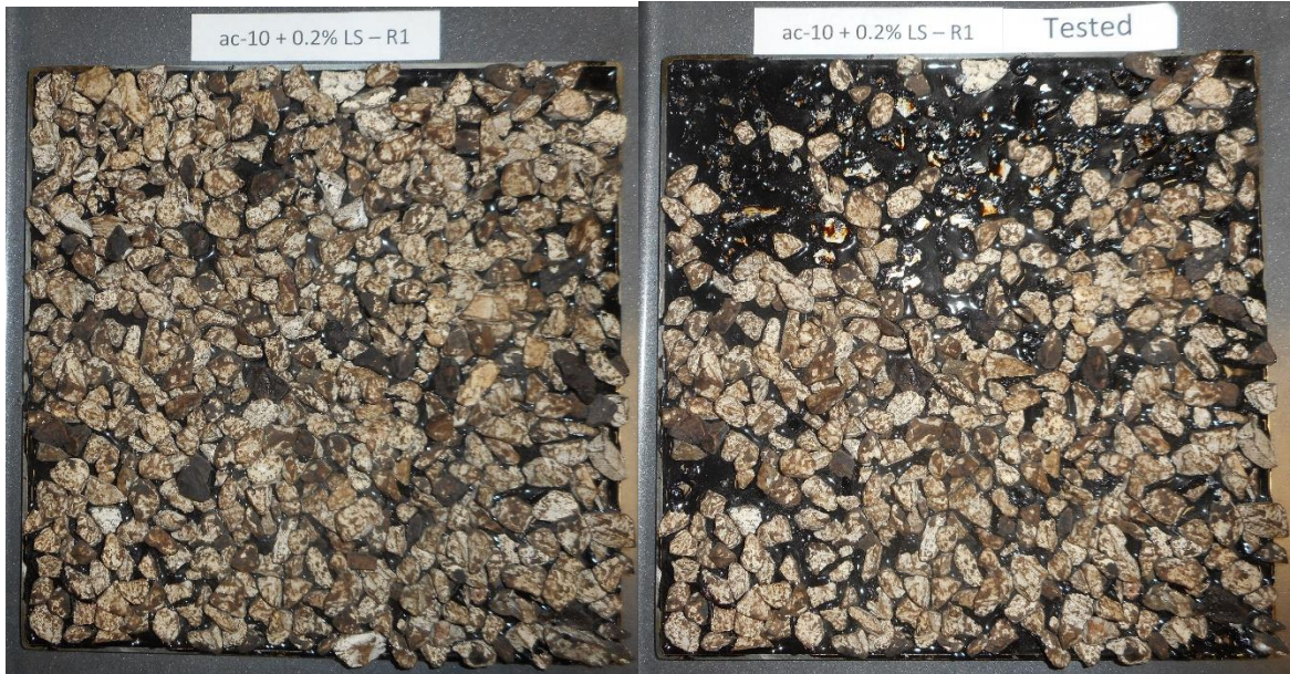
Figure 6. Vialit Plate Before and After Testing.
