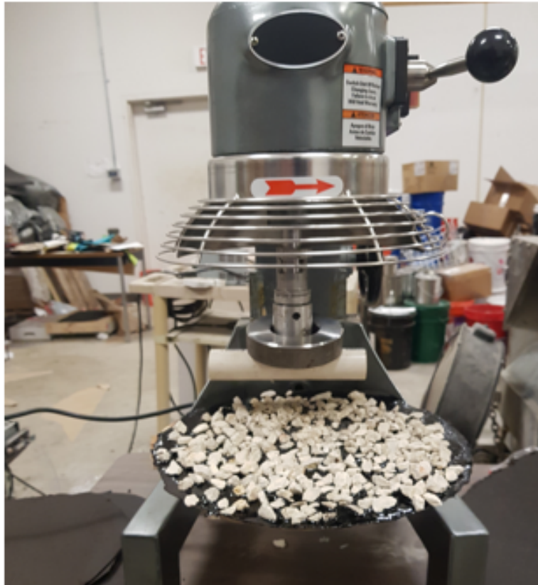
Figure 3.3. Specimen in the Sweep test
