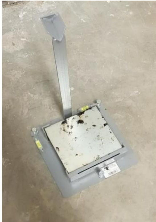
Figure 4 Vialit plate on the 3-point supports.
