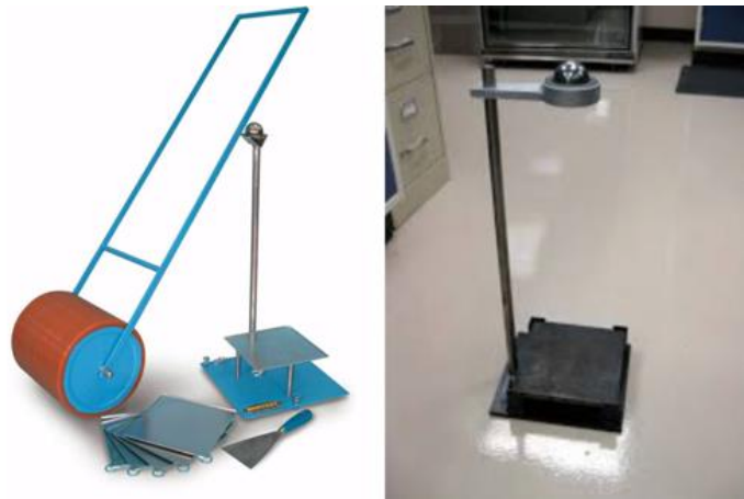
Figure 2.3. A photograph of the Vialit test apparatus (British Standards International)
