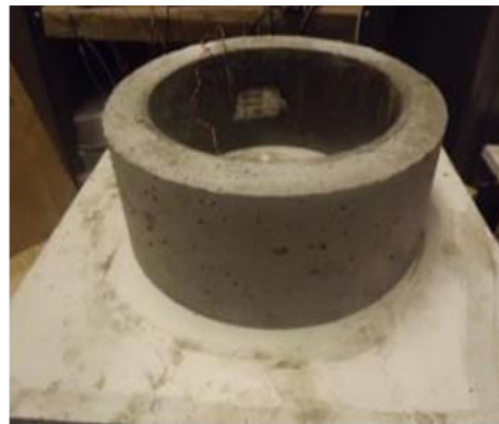
(b) Concrete ring sample
