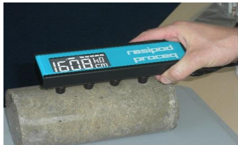
Figure 3.7. Surface resistivity test
