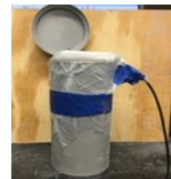
(b) Concrete cylinder with moisture sensor
