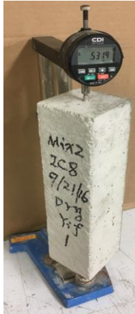
Figure 3.4. Specimen and comparator for free drying shrinkage
