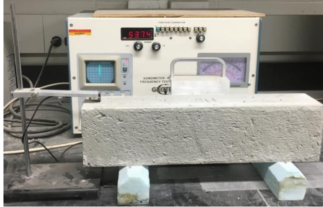
Figure 3.8. Fundamental transverse frequency measurement for dynamic modulus
