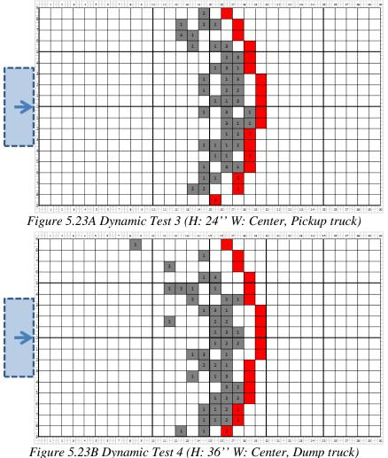
Figure 5.23 HighResolution: Detection Zone Diagram with Pickup and Dump Trucks
