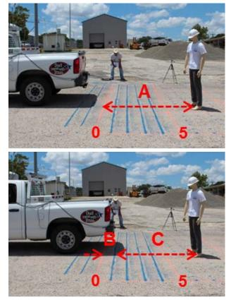
Note: Distance A: Maximum detection range of the sensor in the static condition Distance B: Reduced distance due to the dynamic condition Distance C: Dynamic detection range of the sensor in the dynamic condition Figure A.14 Basic Procedure of the Dynamic Test
