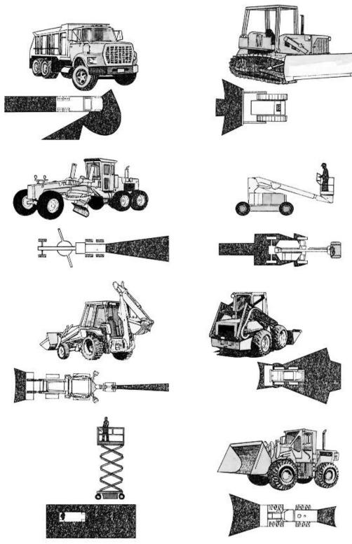
Figure 2.11 Blind Areas around Heavy Equipment (Construction Health and Safety Manual-Ch.28 Backing Up)
