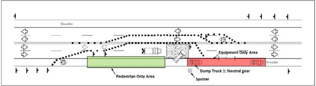
Figure A.7 Detailed IITCP Diagram IV: Vehicle Loading or Dumping
