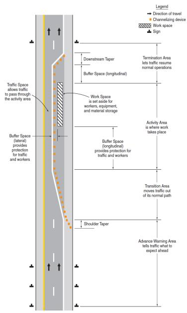
Figure 2.1 Temporary Traffic Control Zone (MUTCD, 2009)
