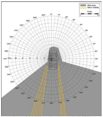
Figure 2.3C 900mm Plane View - GMC 3500 Figure 2.3 Ground Plane, 1500mm Plane, and 900mm Plane Views - GMC 3500
