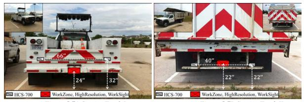
Figure 5.7A Service Truck IFigure 5.7B Service Truck IIFigure 5.7 Sensor Installation Survey on Two Types of Service Trucks
