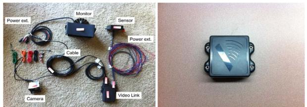
Figure 5.3 HighResolution: Major Component (Left) and a Pulsed Radar Sensor (Right)
