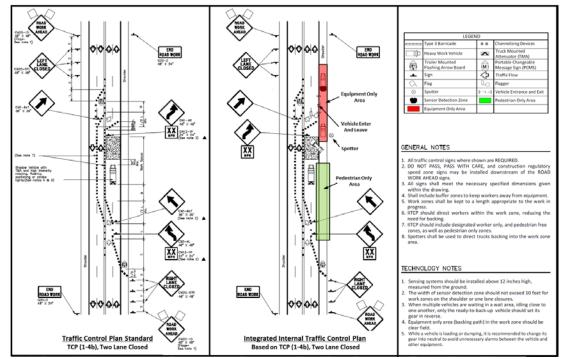
Figure 6.1 A Sample of Integrated and Internal Traffic Control Plan Based on TCP Standard (1-4b)
