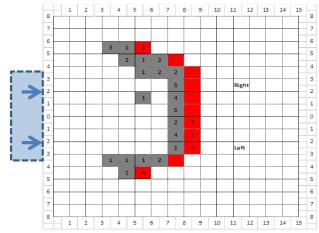
Figure 5.21 HCS-700: Detection Zone Diagram with Pickup Truck
