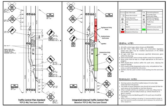
Figure A.1 A Sample of Integrated and Internal Traffic Control Plan Based on TCP Standard (1-4b)
