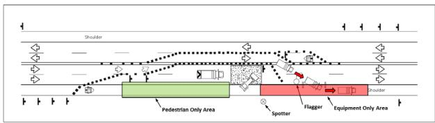
Figure A.2 Detailed IITCP Diagram 1: Vehicle Entering
