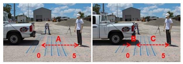
Note: Distance A: Maximum detection range of the sensor in the static condition Distance B: Reduced distance due to the dynamic condition Distance C: Dynamic detection range of the sensor in the dynamic condition Figure 7.5 Basic Procedure of the Dynamic Test
