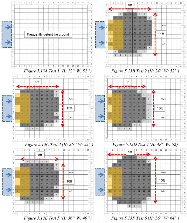
Figure 5.13 HCS-700: Detection Zone Diagram at Six Installation Positions
