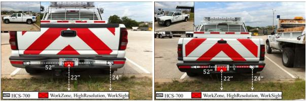
Figure 5.6A Chevrolet-1500Figure 5.6B RAM-1500Figure 5.6 Sensor Installation Survey on Two Types of Pickup Trucks
