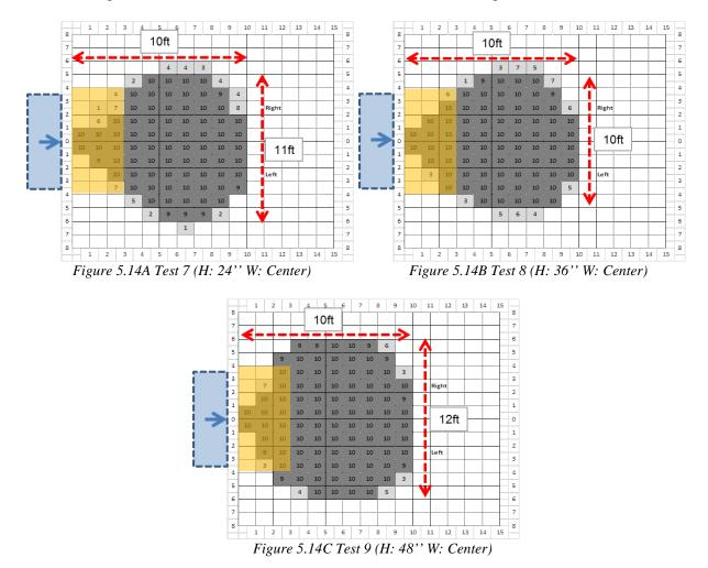
Figure 5.14 WorkZone: Detection Zone Diagram at Three Installation Positions
