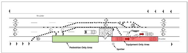
Figure A.8 Detailed IITCP Diagram V: Vehicle Exiting the Work Zone
