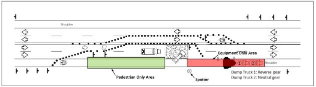
Figure 6.4 Detailed IITCP Diagram II: Vehicle Idling with WorkSight System
