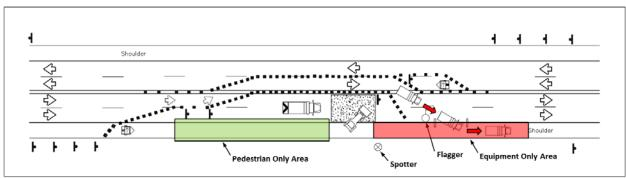
Figure 6.2 Detailed IITCP Diagram 1: Vehicle Entering
