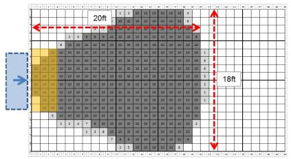
*Figure 5.16C Test 15 (H: 48'' W: Center)* **Figure 5.16 WorkSight: Detection Zone Diagram at Three Installation Positions**
