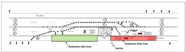
Figure 6.8 Detailed IITCP Diagram V: Vehicle Exiting the Work Zone
