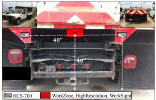
Figure 5.5C F-450 Dump Truck Figure 5.5 Sensor Installation Survey on Three Types of Dump Trucks
