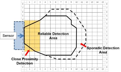
**Figure 7.4 Example of Performance Evaluation Factors in the Static Test**
