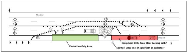
Figure A.5 Detailed IITCP Diagram III: Vehicle Backing
