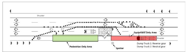
Figure 6.3 Detailed IITCP Diagram II: Vehicle Idling with HCS-700 System
