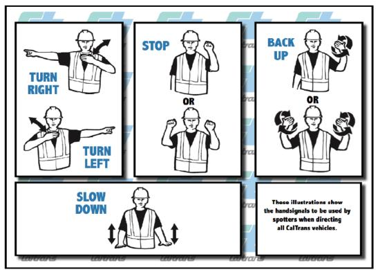
Figure 2.12 Hand Signals Illustration (Cooper et al. 2010)
