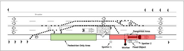
Figure 6.6 Detailed IITCP Diagram III: Vehicle Backing with Fixed Object
