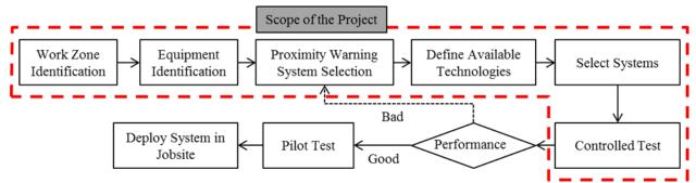
Figure A.10 Process of System Selection
