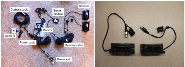
Figure 5.1 HCS-700: Major Component (Left) and Two Ultrasonic Sensors (Right)
