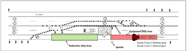
Figure A.4 Detailed IITCP Diagram II: Vehicle Idling with WorkSight System
