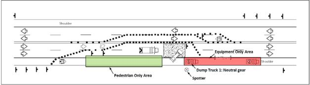
Figure 6.7 Detailed IITCP Diagram IV: Vehicle Loading or Dumping
