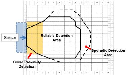
Figure A.13 Example of Performance Evaluation factors in the Static Test
