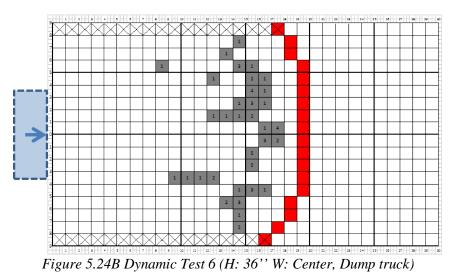
Figure 5.24 WorkSight: Detection Zone Diagram with Pickup and Dump Trucks
