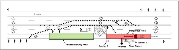
Figure A.6 Detailed IITCP Diagram III: Vehicle Backing with Fixed Object
