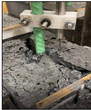
Longitudinal splitting failure (LS)
