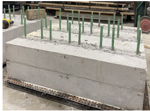
Readied concrete slabs with embedded rebars
