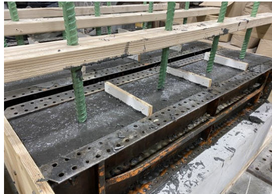
Specimen after pouring UHPC
