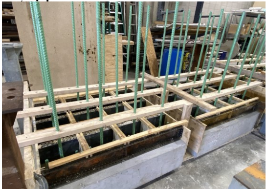
Installing 0.5 in. divider to form discontinuous samples
