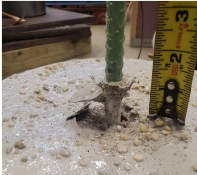
Figure 4. Typical pull-out failure
