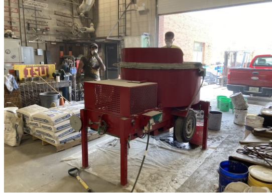
Mixing UHPC constituents using 5 ft 3 mixer
