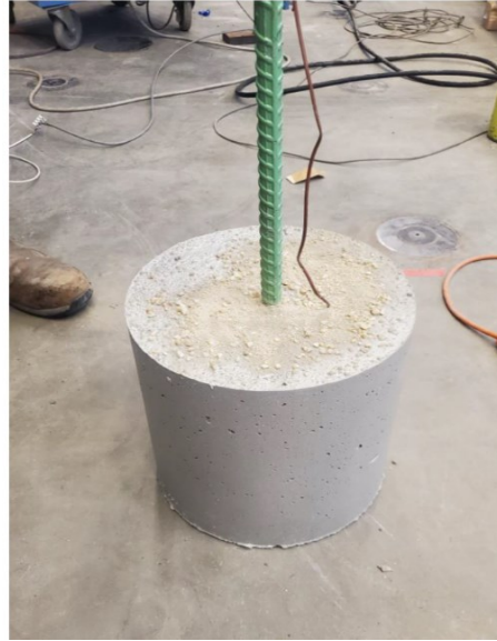
Pull-out test sample after casting
