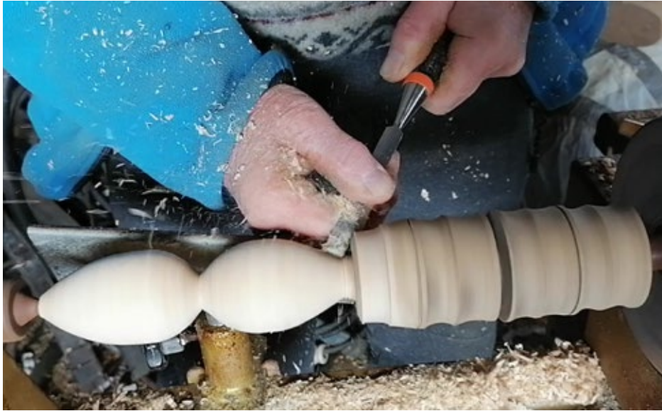
Figure 11. I had the lathe in my workshop at the farm where I also found the piece of wood. I asked my father to help me make some new eggs. My father shows me how to use the lathe to make the new wooden eggs. Photograph: Wenche Sørmo
