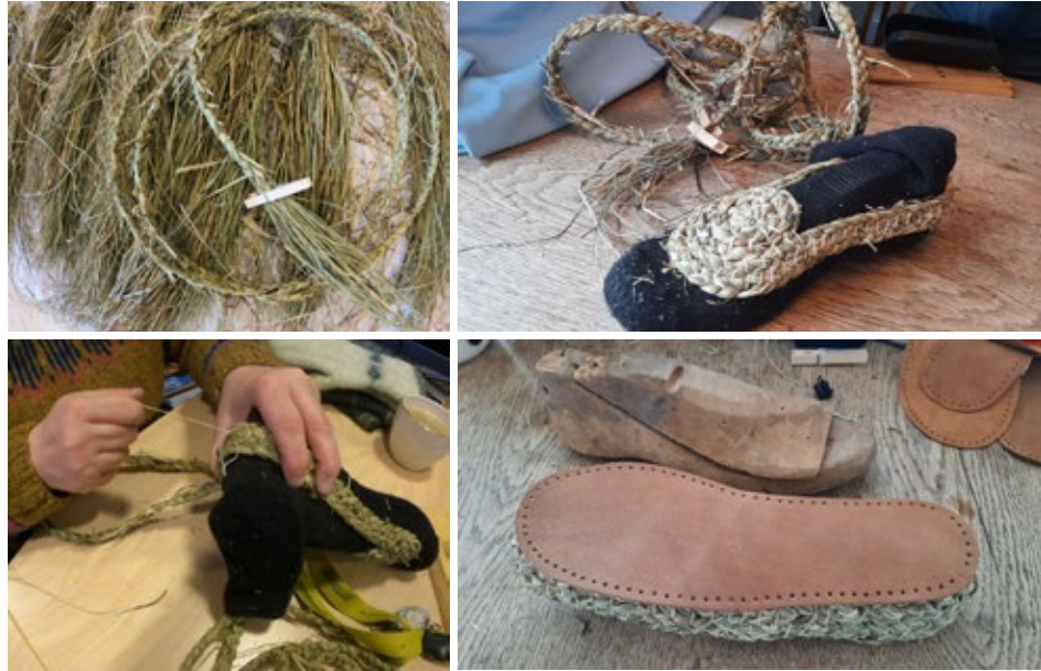
Figure 8. Image series showing the making process. The whole process of making shoes from grass is a multi-sensory experience: the dried sedge has a light gray-green colour, and at the same time it is smooth and strong and smells fresh, with a hint of lemon. When working with it, it is rustling and feeling like hay. Photographs: Karin Stoll
