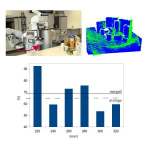
Figure 1: As the camera is moved (left), multiple frames can be captured that cover different parts of the objects in the scene (right), increasing the overall classification accuracy (bottom).
