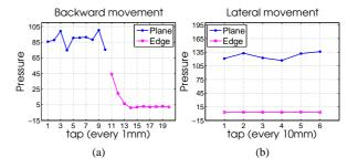
Figure 5: Edge and plane detection in testing phase; (a) back-ward movement, (b) lateral movement.
