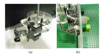
Figure 1: (a) iCub finger mounted on an *xy*-table robot to allow the movement of the finger across a plastic wall (b) to collect data from plane and edge.
