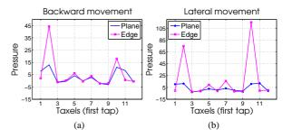
Figure 4: Pressure contact of first tap over plane and edge; (a) backward movement, (b) lateral movement.
