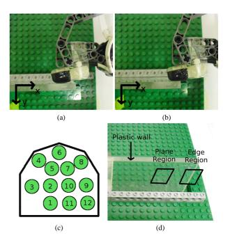
Figure 2: The iCub fingertip moved by the *xy*-table robot; (*a*) tapping in a plane region, (*b*) tapping in an edge region, (*c*) distribution of taxels in the iCub fingertip, (*d*) edge and plane regions. Note the positioning of the fingertip relative to the stimulus.
