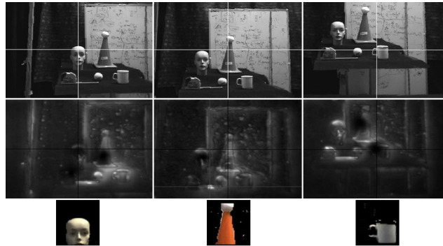
Fig. 6. Sample behavior: (from left) 1. Attention shifts to head from inhibited base of cone, forehead is segmented from background in fovea; 2. Attention returns from inhibited head to top of cone, cone is segmented; 3. Attention shifts from inhibited cone to mug, mug is segmented.
