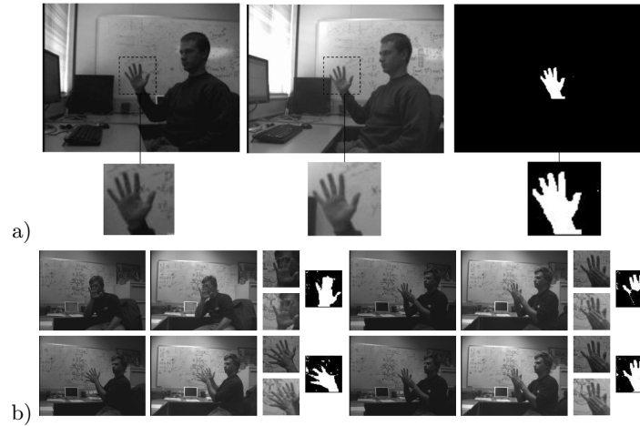
Fig. 2. a) MRF ZDF output (right) with left and right input (respectively) and foveal processing regions. b) Robust performance – segmentation of attended hand from face in near background (top left); a distracting hand (bottom left); and an occluding hand a distance of 3m from the tracked hand 2m from the cameras (top right). If closer than 3m , they are jointly segmented (bottom right).
