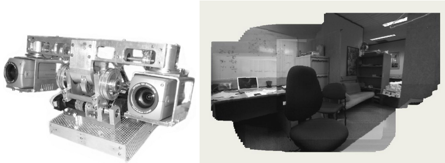
Fig. 1. Left: CeDAR, active vision apparatus. Right: Active rectification mosaic.
