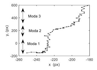
Fig. 6. The movement trajectory of the cube center and three different modes in the image plane coordinates  $\frac{1}{2}$
