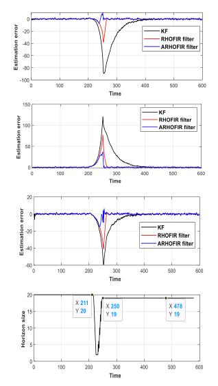
Fig. 3. Dependensies estimation errors for the model state and the horizon sizes on time  ${\bf r}$
