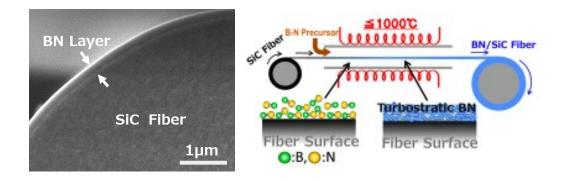
Figure 1 – SEM Photograph of new BN coating on SiC fiber.
