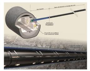
Figure1 the high-level waste repository concept [1]
