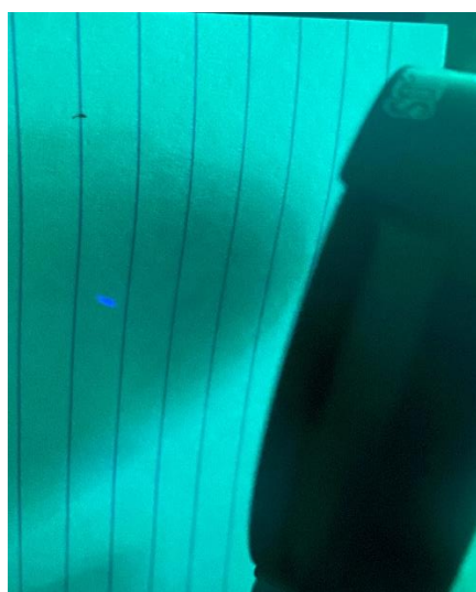
Figure 20: The faint second harmonic spot with the red light filtered out.
