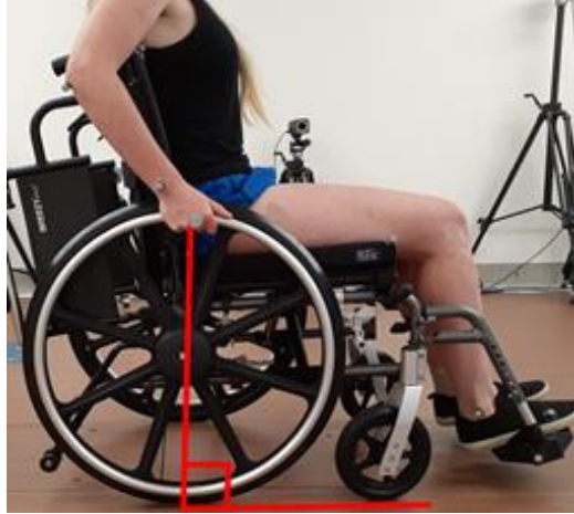
Figure 10: The subject was asked to position their dominant hand at top dead center of their pushrim, so that the reflective marker on their third metacarpal joint aligned with the axle marker, making a perpendicular line with the floor.
