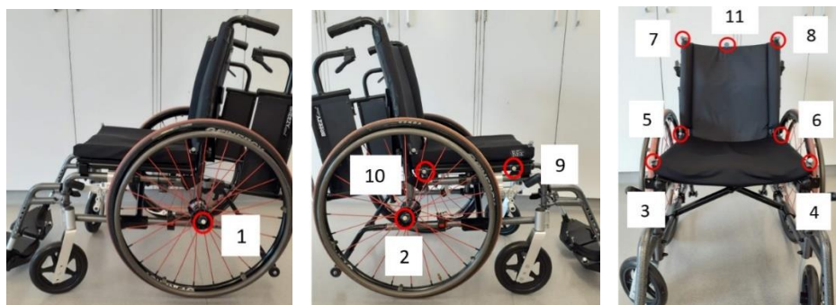
Figure 6: Reflective markers were placed on the 1) left axle, 2) right axle, 3) front right seat, 4) front left seat, 5) back right seat, 6) back left seat, 7) top right backrest, 8) top left backrest, 9) front seat frame, 10) back seat frame, and 11) top middle back rest
