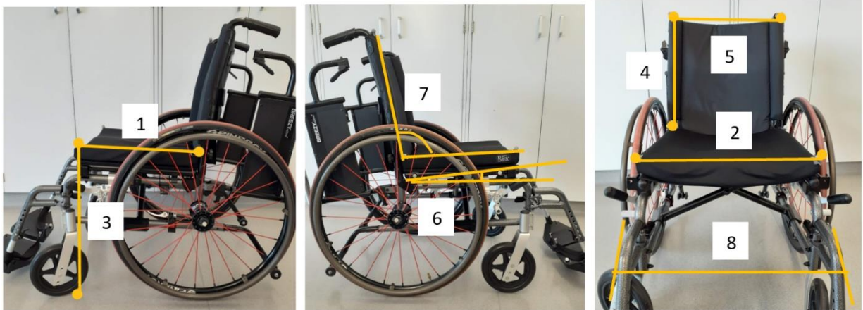
Figure 7: Reflective markers positioned on the wheelchair were then used to find the 1) seat depth, 2) seat width, 3) seat height, 4) backrest height, 5) backrest width, 6) seat sagittal angle, 7) seat to backrest angle, and 8) wheelchair width (distance between left and right axle)
