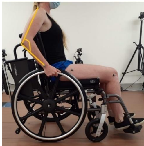
Figure 14: The reflective markers on the acromion process, olecranon process, and ulnar styloid were used to find the sagittal elbow flexion angle, or angle between the forearm and upper arm.
