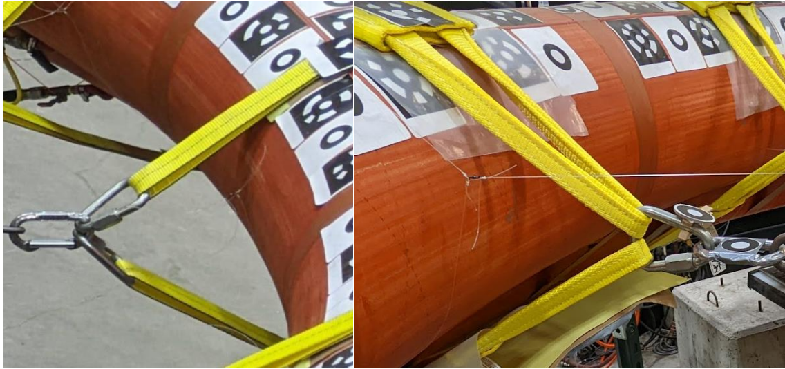
Figure 31. Old (right) and new (left) load cable to strap connections
