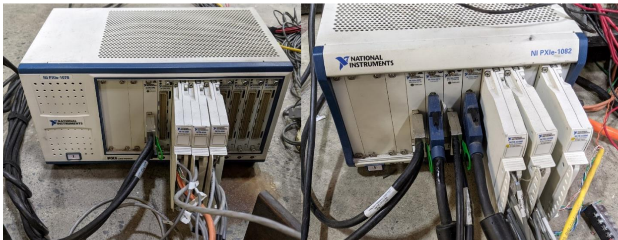
Figure 11. NI PXIe-1078 with TB 4330 cards (left) and NI PXIe-1082 with TB 4339 cards (right)
