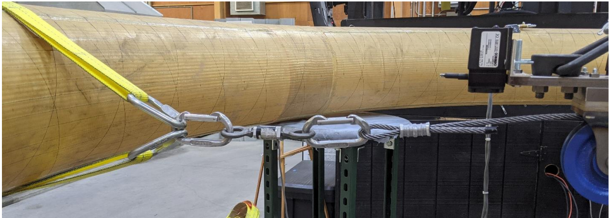
Figure 12. Load cable setup
