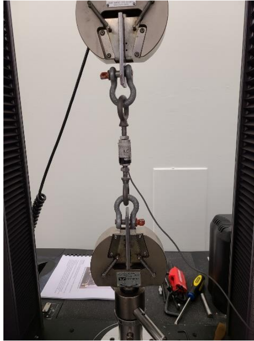
Figure 13. Verification of load cell
