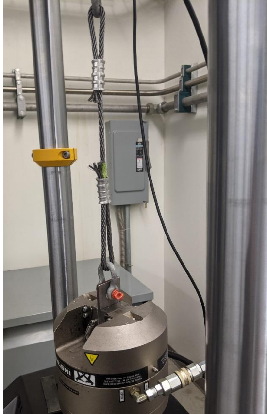
Figure 9. Testing of crimped wire rope
