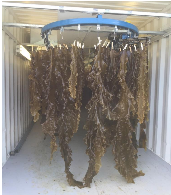
Figure 2.16: Wet kelp in the drying chamber to start the drying process.
