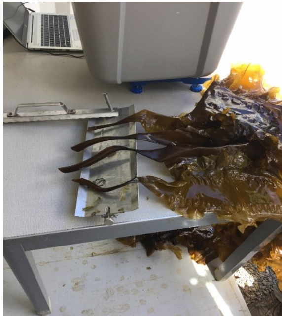
Figure 2.14: Wet sugar kelp laid out to be attached to a custom seaweed hanger.
